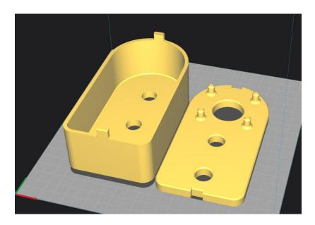
Layer Height: 0.2 Wall thickness: 1.2mm Bottom Layers: 4 Top Layers: 4 Infill type: cubic Infill Density: 15% Support: no
